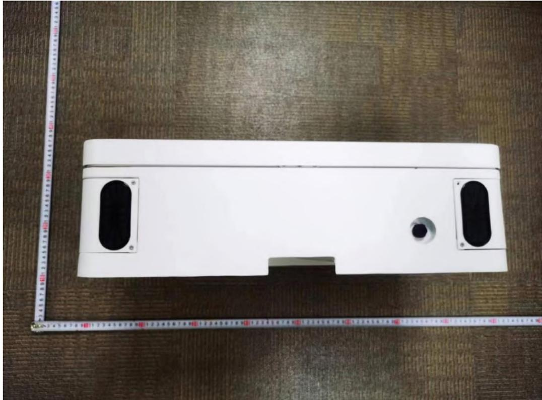
Main control unit, Model: TBMS-MCS0800 (Back view)
